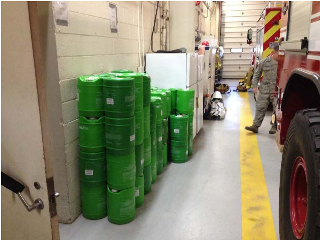
Photo 2: View of Firestation #1. 5 gallon buckets of AFFF.
